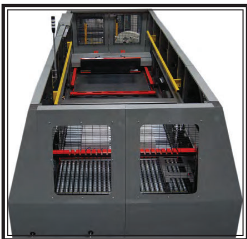
View of Upper Palletizing Section
